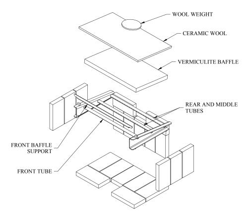
Figure 4.6.1 (A) – Baffle installation for Escape 1800
